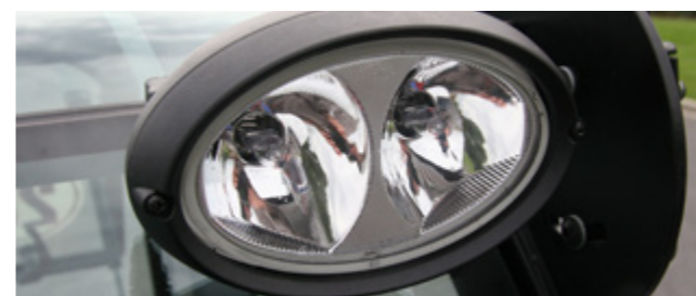
2x Dual Power working lamp front, 1x Single Power rear
