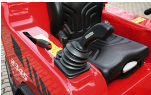
The slightly twisted joystick position simplifies operation.
