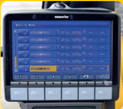
Komatsu Integrated Attachment Control (KIAC) for up to 15 tool presets for oil flow and pressure (option)
