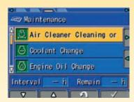
The multifunction monitor panel provides the operator with maintenance and service information.
