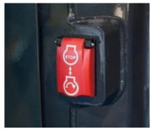
Secondary engine shut down switch
